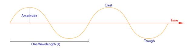
This means that a microwave oven has hot spots where there are crests and troughs and cold spots in between. Part of this issue is remedied by the use of a mechanical turntable that rotates the food through the hot spots and results in more even overall heating.
